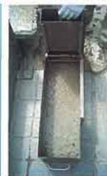
鉄筋格子付L型試験器 L-shape Flow Test with a Steel Bar Mesh Gate
